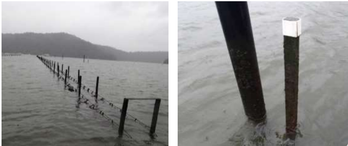
Figure 1: Oyster farm system deployed in the Hawkesbury river estuary, Mooney Mooney, NSW, Australia (left), and one of the eight Accoya Radiata pine stakes installed in the field trial (right).
